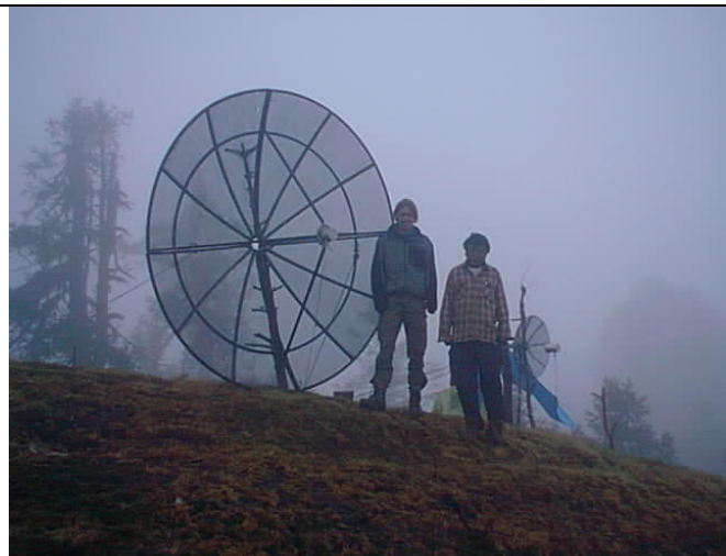
The first long range link testing (34 KM) was done in 2002 from Mohare to Pokhara putting a dish on the ground
