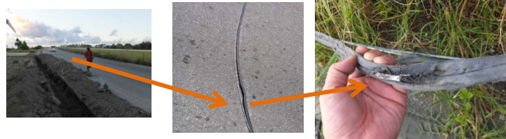
Crossing the fiber cable on the main road in hot days, the cable was destroyed.
