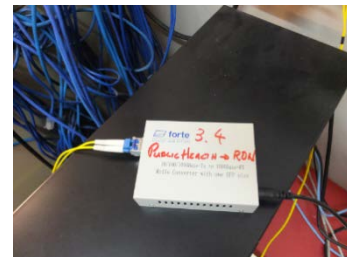
Terminal box and Media convertor at the end user premises.
