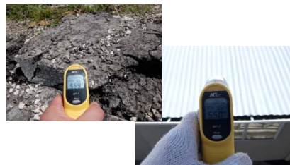
Measured temperature on road and roof * about 56 degree
