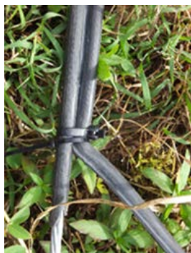
Trouble at the 1 st practice (broken all fibers )
