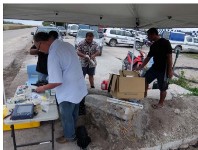
Measuring the length and break point by OTDR (filed check at fusion splicing point)
